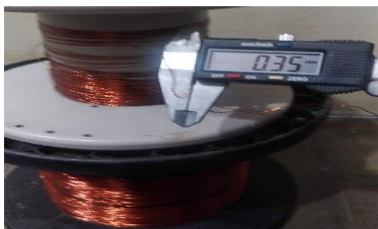
Figure 6. Measuring the diameter of copper wire
