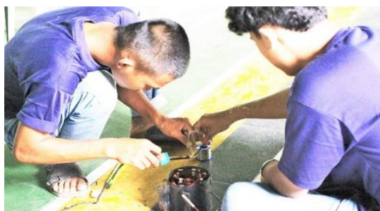
Figure 11. Splicing the coil winding with solder
