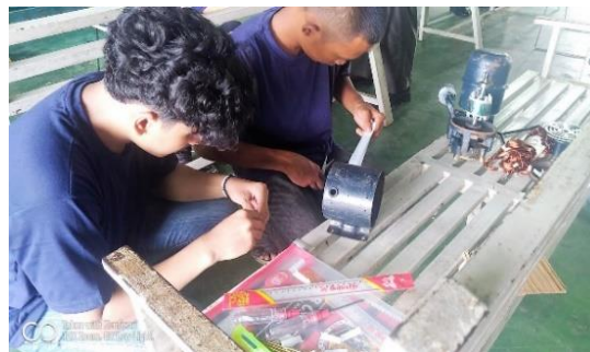
Figure 8. Installing the winding sleeve on the Cern
