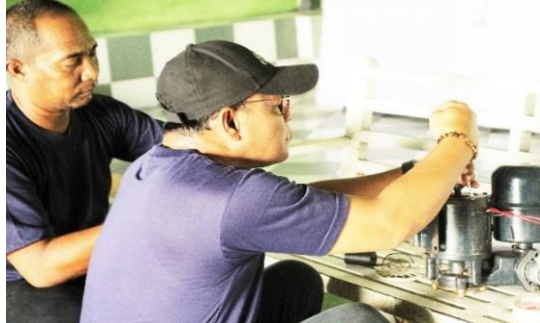
Figure 12. Re-covering the motor that is ready to roll
