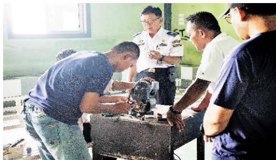
Figure 13. Testing the pump motor that has finished rewinding the coil winding
