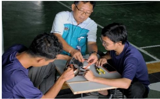
Figure 10. Installing the winding into the Cern groove of the electric motor
