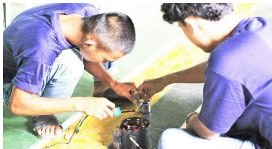
Figure 11. Splicing the coil winding with solder
