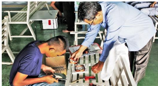
Figure 5. Making the coil winding of the water pump motor
