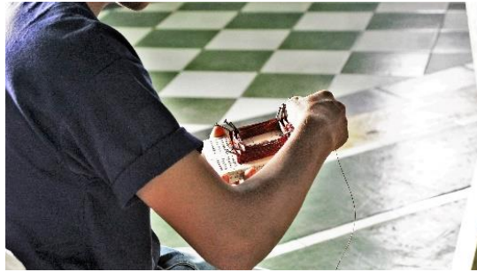
Figure 9. Rolling the coil onto the mull board
