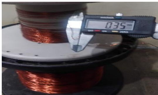
Figure 6. Measuring the diameter of copper wire
